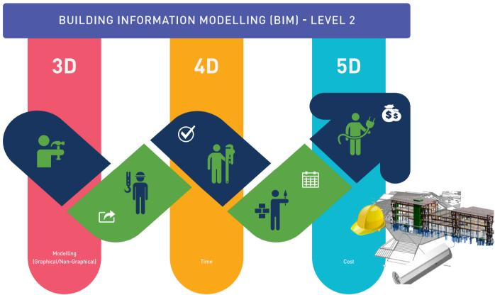
Setting the foundation for design to build projects like the Coca Cola Arena, BIM 5D is becoming the norm. BIM is comprised of a 3D Graphical Representation of the Structure + 4D Construction Schedule (sequencing, visual depiction, resets based on plan versus actual) + 5D Cost Data (for cost estimation on bids, purchasing, installing, operating, maintenance – cost is continually updated compared to plan).
